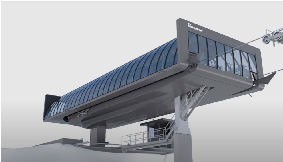
Figure 9: A standard 3D view of a Doppelmayr D-line top station
